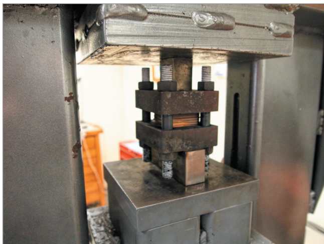
Figure 16 25% hot press reduction
