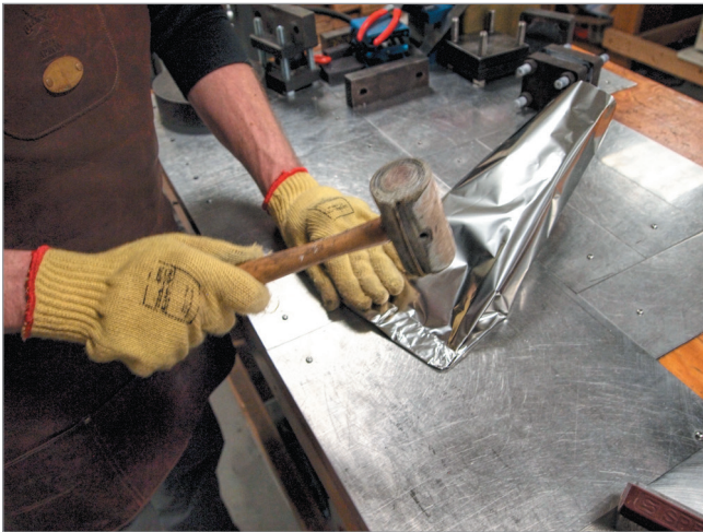
Figure 12 Rawhide mallet being used to seal bag end
