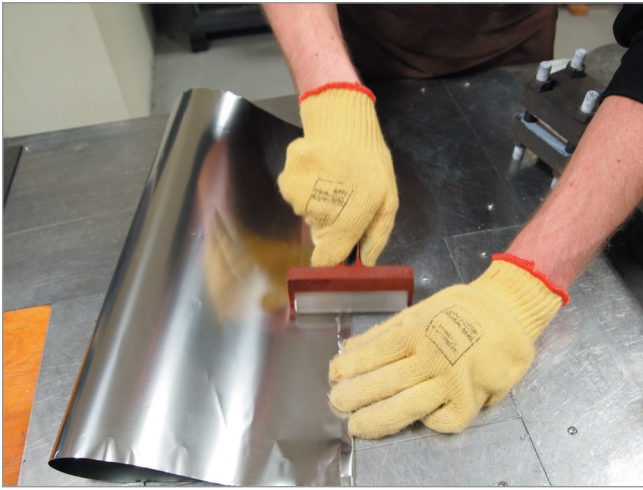
Figure 11 Using acrylic roller to make flat seams in stainless foil to create a bag
