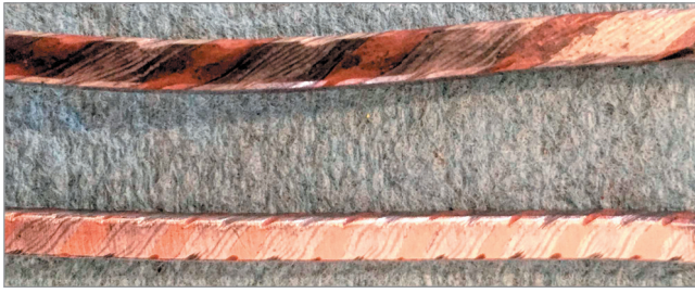
Figure 25 Loose- and tight-twisted square stock
