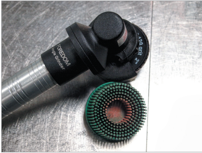
Figure 22 3M Roloc bristle disc and ForeDOM angle-grinder attachment
