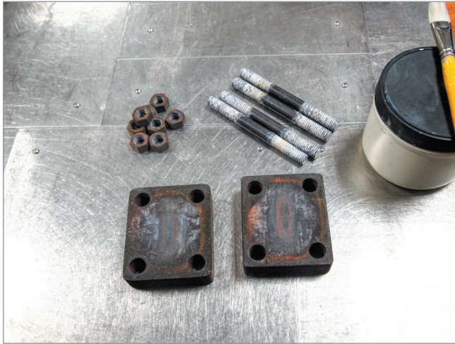
Figure 7 A-286 torque plates and 718 bolt studs
