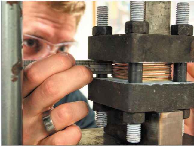
Figure 10 Aligning metal using a straight edge prior to tightening torque plates
