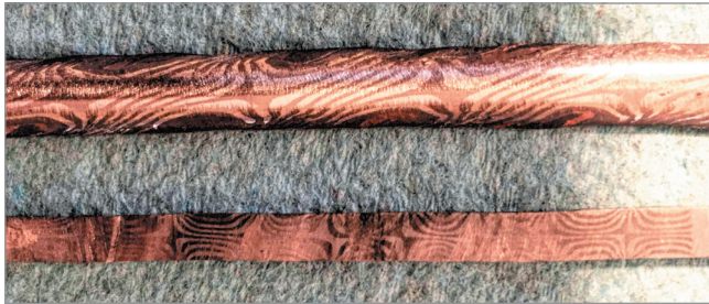
Figure 26 Loose (top) and tight (bottom) star patterns
