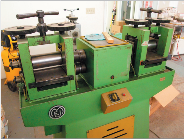
Figure 17 Rolling mill (Don't put your hand in here; it hurts!)
