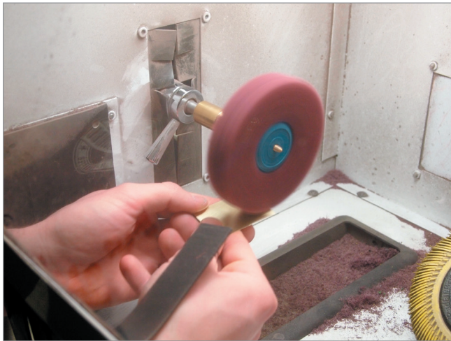
Figure 5 Cleaning metal with a Scotch-Brite™ buff
